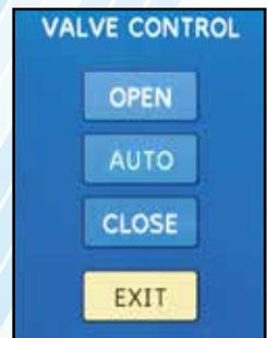
The control valve can be quickly set in OPEN, CLOSE or AUTO mode.
