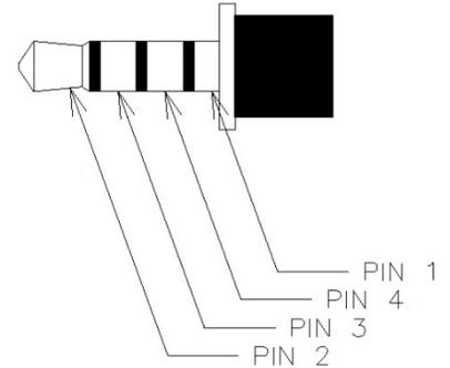
If making up a cable to interface from the TRRS 3.5 mm jack connector to a standard PC 9-pin serial port (RS232), use the connections as listed here.
